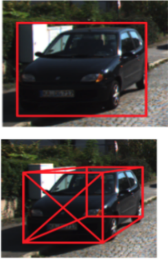
Fig. 1. Deep3DBox [7], one of the methods that performs 3D object detection using a single RGB image.
